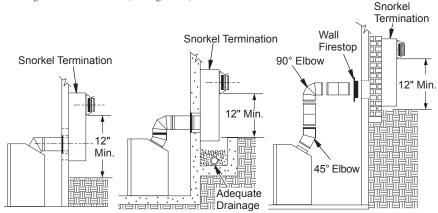
Figure 16 - Snorkel Termination Configurations for Below Ground Installation
